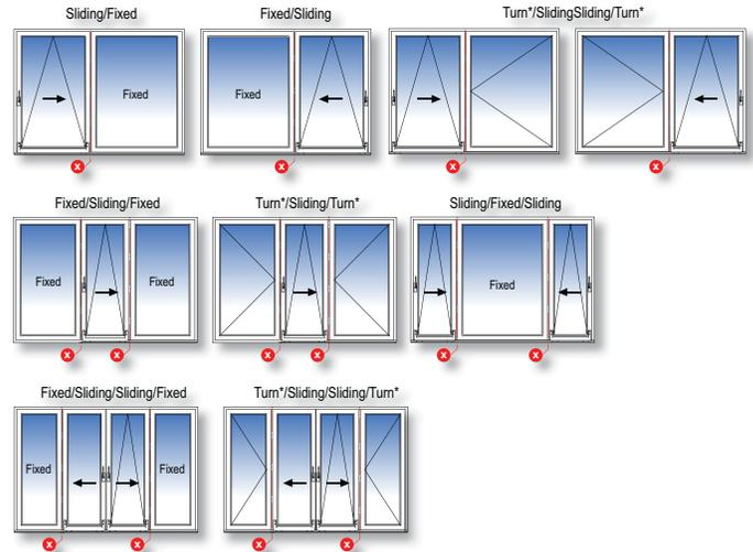
\* Turning sash only with removable handle. Depending on hardware manufacturer different opening types available.
